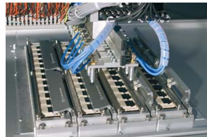
Close up view of the 48 contact pads. The exchangeable contact pads are currently available for SD Card/MMC, RS-MMC and microSD memory media.
