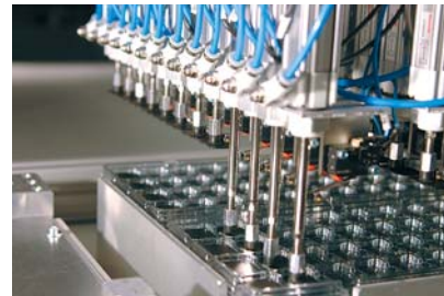
The robot arm picks up the memory cards using suction pads.
