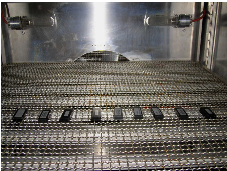
Location of the test item(s) in the Climate Chamber (passiv)
